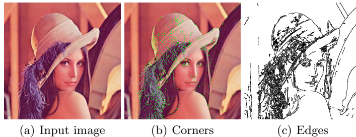
Fig. 3. Edges and corners detection within our framework
