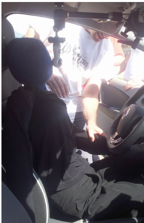
Figure 3: Installation of the soft dummy and the 360° camera within the autonomous car.
