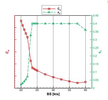
Figure 11: Drag  $C_d$  and transition point location  $x_{tr}$  for the flexible hydrofoil as functions of the boat-speed (BS).
