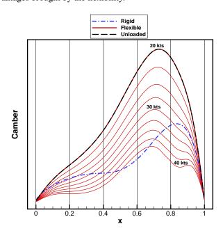
Figure 7: Flexible hydrofoil camber distribution at several boat-speeds. The rigid hydrofoil case is also shown for comparison.
