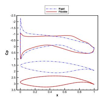
Figure 4: Shapes and distributions of Cp at 20 kts of boat-speed for the rigid and flexible hydrofoils.
