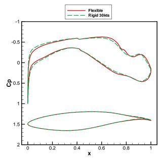
Figure 12: Shapes and pressure coefficient Cp distributions for the flexible and Rigid 30 kts solutions at 30 kts of boat-speed.
