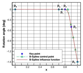
(a) B-Spline approximation of the rotation angle.
