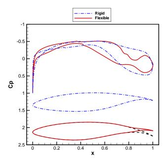
Figure 5: Shapes and distributions of the pressure coefficient Cp at 40 kts of boat-speed for the rigid and flexible hydrofoils.
