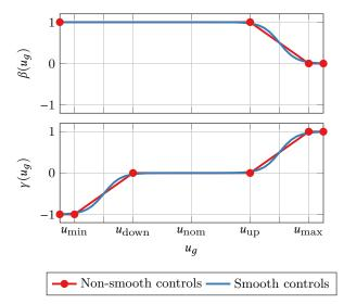
Figure 2: Local control functions used for the feed-back controls. Smooth functions for P(U) and Q(U). Non-smooth functions for the "AMI-based deed-back" control.
