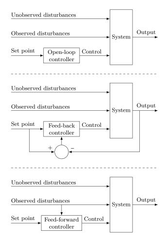
Figure 1: open-loop, feed-back and feed-forward control.
