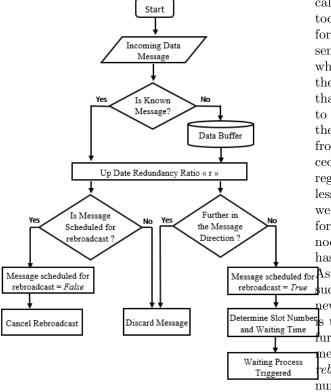
Figure 2: Flow chart of Reception Procedure for SEAD2 Protocol
