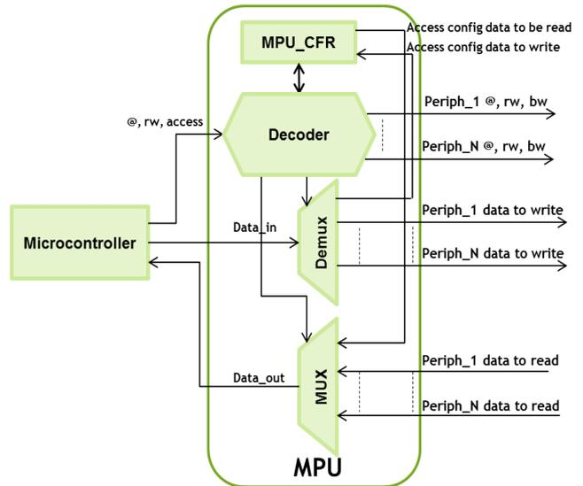
Figure 3: MPU architecture
