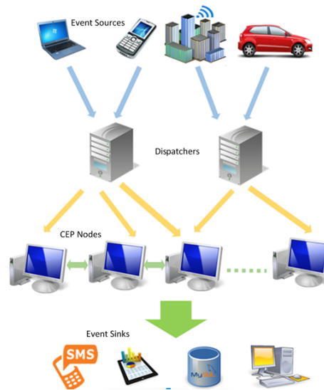
Fig. 1. VISIRI high level architecture
