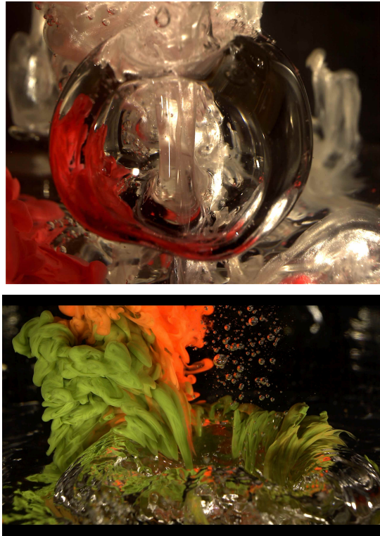
Fig. 11. Several examples of interaction between a bubble created by an air gun bullet and injected color paints.
