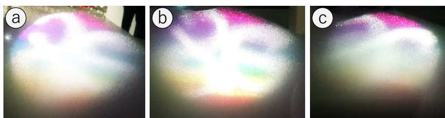
Fig. 10. 3D form display composed of bubble cluster. Photo from the (a) left, (b) front, (c) right (projecting the inverted ace2016 logo).
