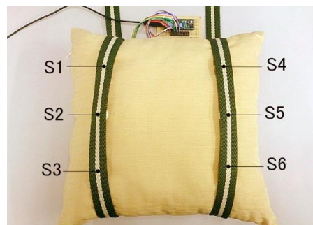
Fig. 5. A cushion equipped with two photo reflective sensor modules.
