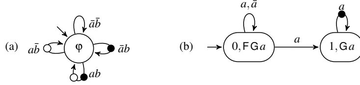
Fig. 1. (a) A TGBA recognizing the LTL property \varphi = GFa \wedge GFb with acceptance conditions \mathcal{F} = \{\bullet, \circ\} . (b) A TGBA recognizing the LTL property \varphi = FGa with \mathcal{F} = \{\bullet\} .
