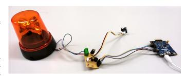
Fig. 2: SAMR21-xpro with custom break-out board connecting light sensor, sound level sensor, buzzer and revolving light.
