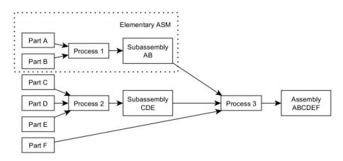
$\textbf{Fig. 2.} \textbf{Example of an assembly situation model for a six part assembly. The dotted portion shows an elementary ASM$
