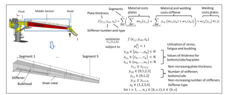
Fig.5. Illustration of a maritime crane box type boom, cost optimization problem and related formalized objective function
