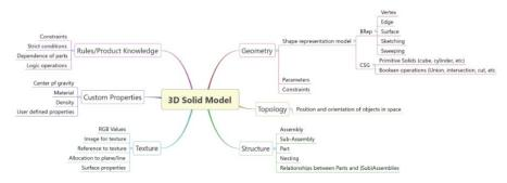
Fig. 2. Type of information embedded in CAD Models
