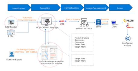
Fig. 1. Use-case scenario: acquiring, formalizing and re-using knowledge for 3D configurators
