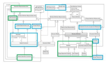
Fig. 8. CAD-KBE-PLM Integration Schema from [6]
