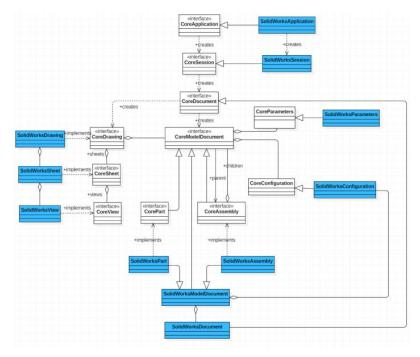
Fig. 5. Core Application implementation in SolidWorks
