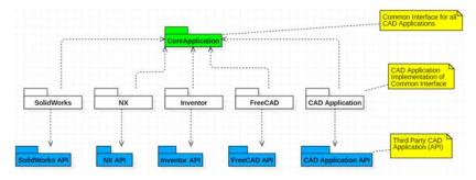
Fig. 4. Modular architecture for Multi-CAD API
