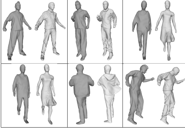
Fig. 6. Examples of changing the clothing dynamics. The meshes in brighter gray are not seen in the training data. They are generated by feeding the motion parameters of the darker gray meshes on the left to the neural network trained on the sequences containing the brighter gray clothes.
