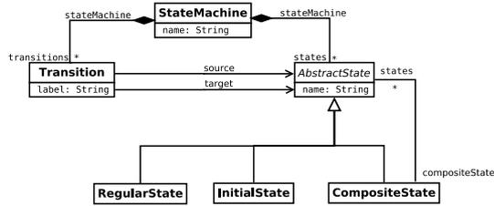
**Fig. 1.** The hierarchical and flattened state machine metamodel
