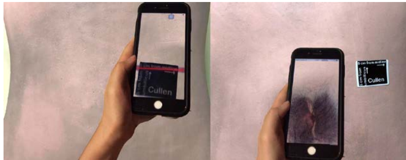
Fig. 1. Using CAROPE: LEFT: marker/trigger (black box) is scanned (red line). RIGHT: Cullen’s sign appears as an AR visual overlay on abdomen of a mannequin.
