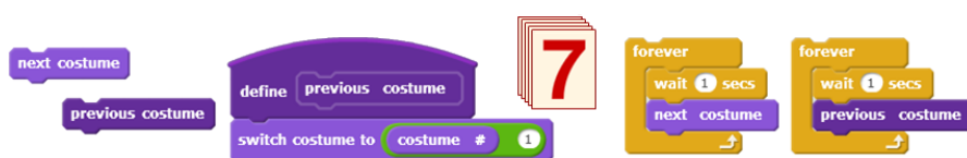
Fig. 7. Patching the language. While next costume is a standard block, ‘symmetrical’ previous costume block can be defined to highlight the analogy.
