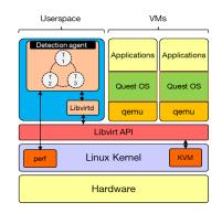
Figure 1: Detection module architecture
