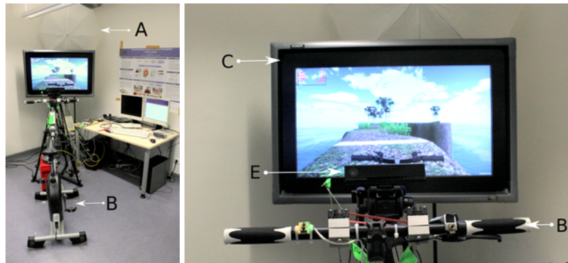
Fig. 2: Hardware Setup of the EmotionBike: Face Illumination Lamp (A), Cycling Game Controller (B), Screen (C) and Camera (D)
