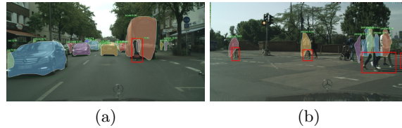
Fig. 7: Failure modes of mid-term prediction with the F2F model, highlighted with the red boxes: incoherent masks (a), lack of detail in highly deformable object regions, such as legs of pedestrians (b).
