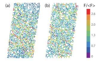
FIG. 1. Examples of an experimental (a) and numerical (b) force network. Experimental and numerical examples are generated at the same strain amplitude  $\gamma=14.9\%$  and  $\phi=0.8036$ . The color scale represents the total force at each contact, normalized by the concurrent mean force. As described in the text, the simulation results in this and all the following figures include additional noise of amplitude 0.01 N, except if specified differently.
