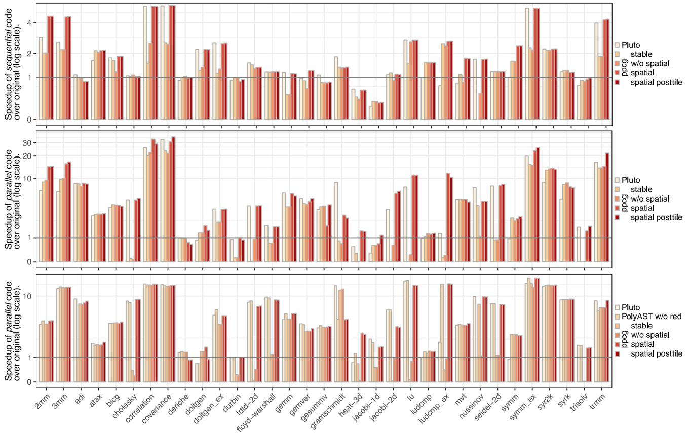
**Figure 1.** Speedup of the optimized tiled code over the original code with different scheduling algorithms; top: sequential code on **skylake**, middle: parallel code on **ivy**; bottom: parallel code on **westmere**.
