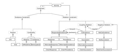
Fig. 1: The declarative process model's hierarchy of constraints. Taking into account the UML Class Diagram graphical notations, the Generalization ("is-a") relationship represents the restriction. The restricting is on the tail, the restricted on the head. The Realization relationship indicates that the constraint template (as well as the restricting ones) belong to a specific type. Constraint templates are drawn as solid boxes, whereas constraint types' boxes are dashed.
