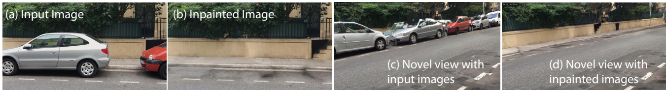
Figure 1: Our multi-view inpainting method can remove objects such as cars (b) from all input images (a) of a multi-view dataset for Image-Based Rendering (IBR). This allows more flexible usage of IBR: by removing the cars, we avoid problems due to bad reconstruction which are more visible in novel views (c-d). Our method preserves perspective cues and provides clean separation between different planes (e.g., wall and sidewalk).
