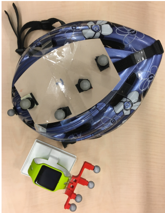
Figure 2: The bike helmet and smartwatch with four markers.
