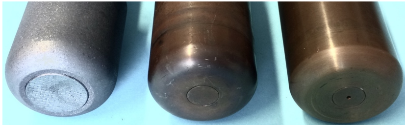
Figure 1: ESA standard probes (5 cm diameter) used for the measurements performed in the Plasmatron facility: (left to right) stagnation-point probe holding a material sample, copper calorimeter, and water-cooled Pitot probe.
