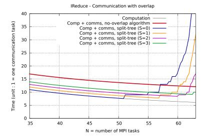
Figure 3: Model of communication/computation overlap for operations constant-size buffer (broadcast, reduce) on 64 cores.
