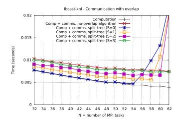
Figure 5: Result of split-tree algorithm with different values of S, for MPLIbcast with constantsize buffer of 2MB on 64 cores (KNL).
