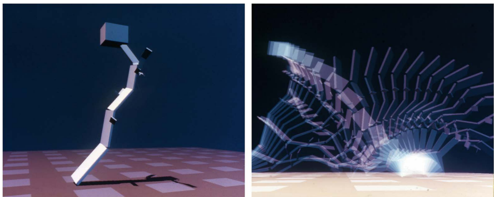
Figure 1. Exploiting potential energy to locomote. Evolution discovers that it is simpler to design tall creatures that fall strategically than it is to discover active locomotion strategies. The left photograph shows the creature at the start of a trial, and the right photograph shows snapshots of the figure over time falling and somersaulting to preserve forward momentum.
