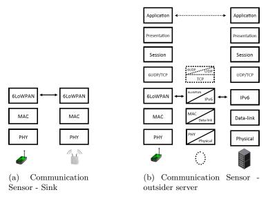
Fig. 4. Type of communication based in layers.
