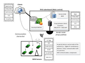
Fig. 5. Representation of one communication ent-to-end
