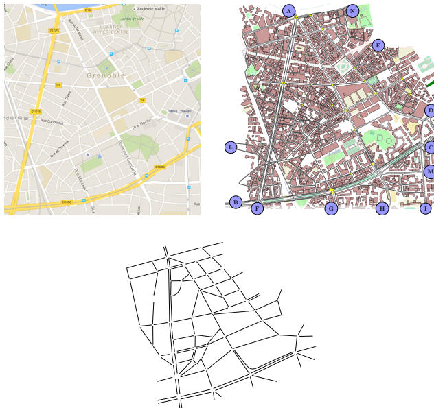
Fig. 10: From top left, clockwise: a map of Grenoble downtown; the corresponding Aimsun model used in the microscopic experiments, with markers for the detector positions that correspond to the inflows of the model (see also Figure 11); the directed graph describing this road network. A demo of our experiments is available online [39].
