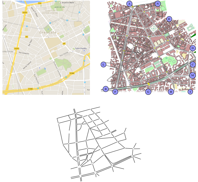
Fig. 10: From top left, clockwise: a map of Grenoble downtown; the corresponding Aimsun model used in the microscopic experiments, with markers for the detector positions that correspond to the inflows of the model (see also Figure 11); the directed graph describing this road network. A demo of our experiments is available online [39].
