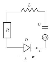
(b) Circuit with an ideal diode and a voltage source.
