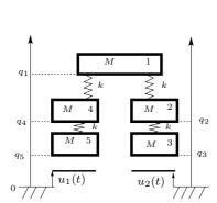
(a) A mechanical system with two unilateral constraints .
