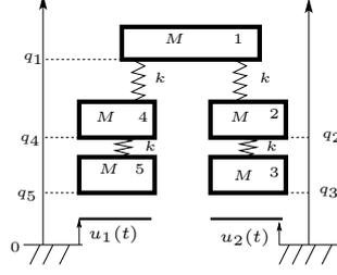
Figure 1: A mechanical system with two unilateral constraints.
