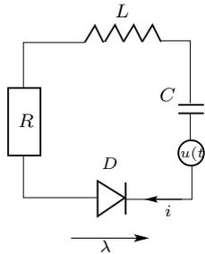
Figure 2: Circuit with an ideal diode and a voltage source.
