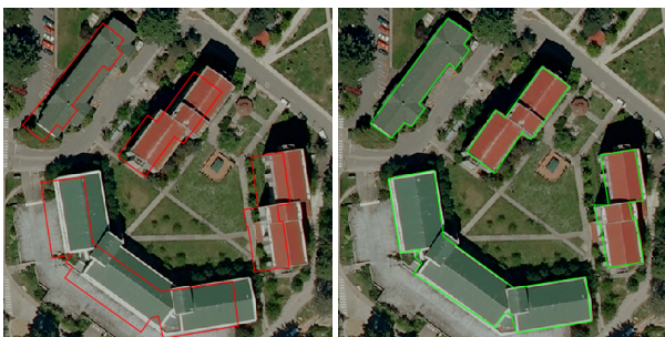
Figure 1. Multimodal matching. We align aerial images with cadastral images. Left: original misregistered images, right: after their realignment.
