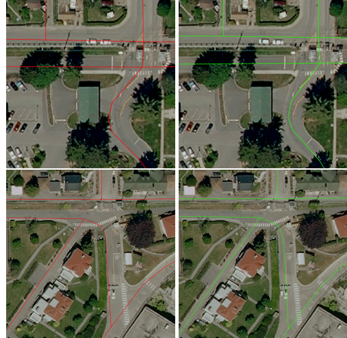
Figure 8. Example of road alignment. Left: original alignment between image and roads (Kitsap); right: results after realignment.
