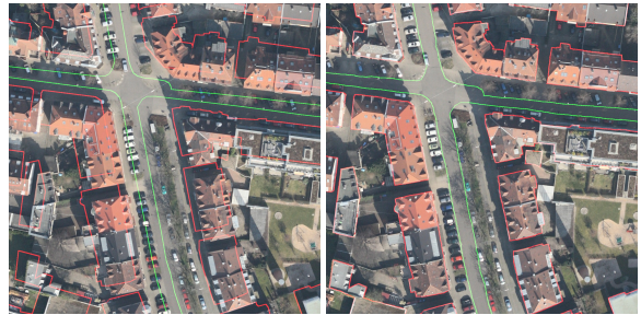
Figure 9. Example of alignment on the Kitti Dataset. Left: before alignment; right: after alignment.
