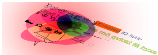
Figure 2: Example of a rendered picture following the canvas fingerprinting test instructions.
