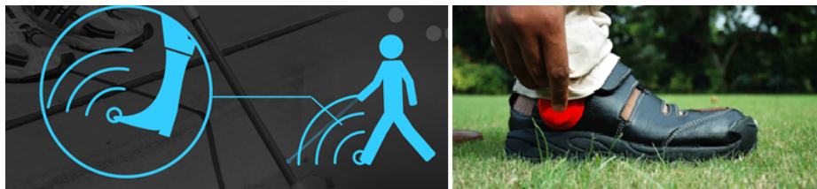
Fig. 1. Depicts Ultrasound sensor that detects the obstacles (left). Depicts design of
