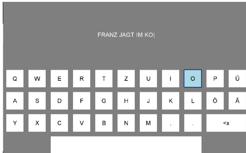
Fig. 1. Screenshot of the implemented on-screen keyboard. Gaze highlighted keys in light blue while a combination of pupil deviation criteria and fixation duration selected (highlighted by a dark blue frame).
