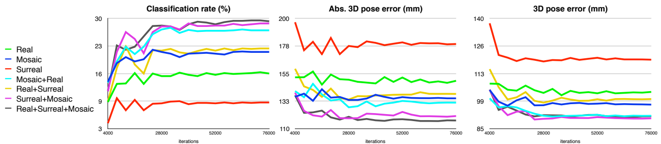
Fig. 7 Human pose estimation results on Human3.6M when training the classifier with different combinations of real, surreal and mosaic data. We report classification rate, absolute 3D pose estimation error and 3D pose error after rigid alignment. We show the performance with respect to the number of training iterations. The three sets of training images all correspond to the same 190,000 3D poses and are labelled with the same class labels.
