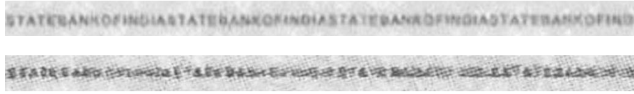
Figure 4. Microlines on genuine (top) and printed checks (bottom).
