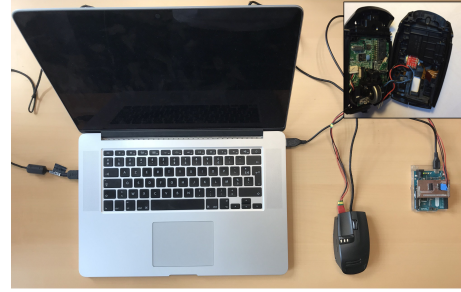
Figure 2: Our setup comprises a Logitech G9 Laser Mouse connected via USB to the host computer with the MPU-9250 chip embedded inside. The MPU-9250 chip is connected to an Arduino Leonardo that is connected to the host computer via USB.
