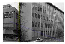
Figure 4: Sample matching points (in blue) from two different images (separated by the yellow marker) that were pruned.
