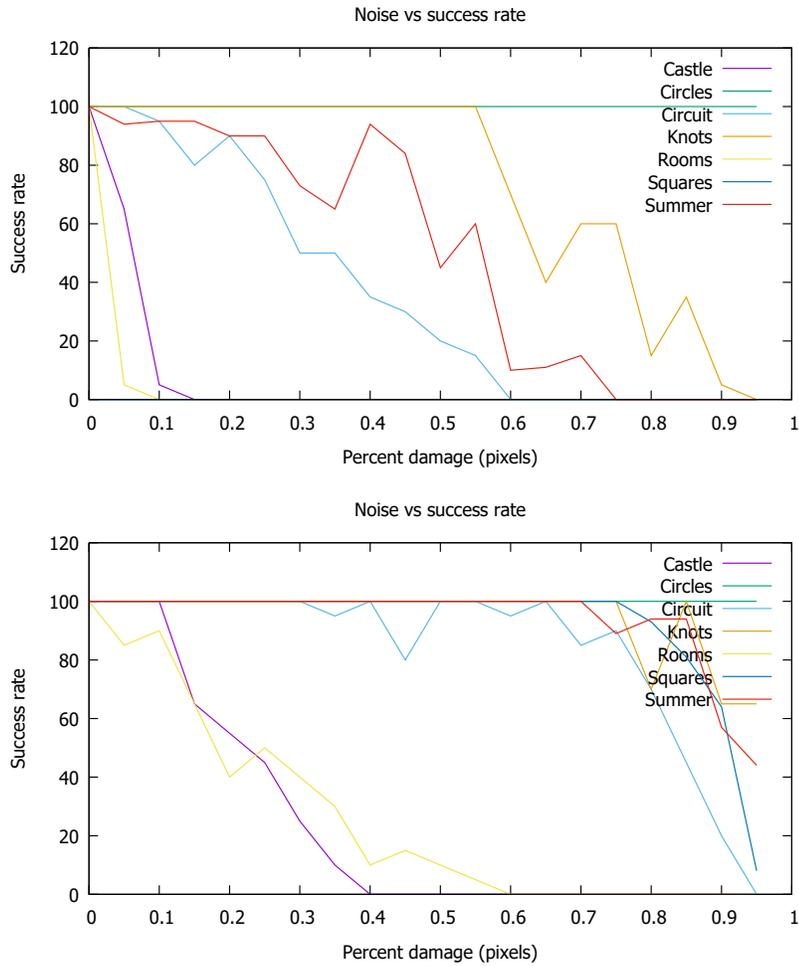
Figure 2: Robustness to noise, plotting decoding success rate versus amount of noise. A percentage of pixels is selected and erased by a random color, with 1 meaning 50% of pixels damaged. **Top:** simple selection of the best matching tile. **Bottom:** robust scheme exploiting constraints.
