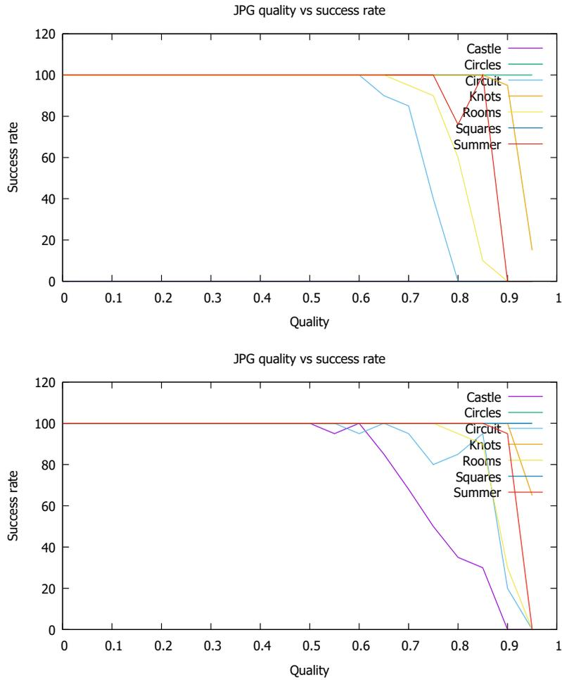
Figure 1: Robustness to jpg compression for various tilesets, plotting decoding success rate versus jpeg quality (0: lossless, 1: maximum compression, using libjpeg setting). **Top:** simple selection of the best matching tile. **Bottom:** robust scheme exploiting constraints.
