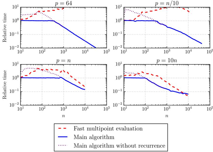
FIG. 2. Performance comparison of various methods to evaluate  $(P_n(x), P'_n(x))$  to  $p$ -bit precision for a set of  $n/2$  points  $0 < x < 1$  distributed like the roots of  $P_n$ . The  $y$  axis (relative time) shows the time divided by the time using the three-term recurrence in fixed-point arithmetic.
