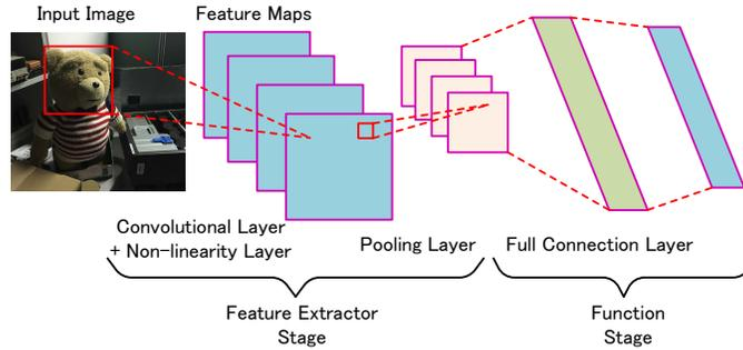
**Fig. 1.** A typical convolutional neural network structure
