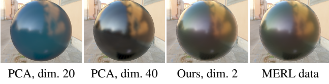
Figure 8: Comparing our method to the “kernel trick” when reproducing input BRDF data for a material in the MERL database ( color-changing-paint3 ). Our method always perfectly reproduces the training materials, regardless of the dimension of the parameter space; this is not the case for kernel approximations (here, using 20- and 40-dimensional PCA approximations).
