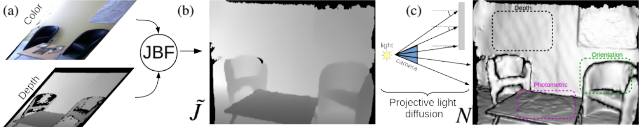
Figure 1. Filtering/fusion pipeline; (a) Raw depth image and RGB image, (b) reconstructed depth image and (c) projective light diffusion image. Emergent depth, photometric and surface orientation scene characteristics captured by PLDI are partially highlighted for emphasis (best viewed in color).
