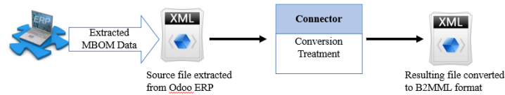
Fig. 5. Global architecture of the connector
